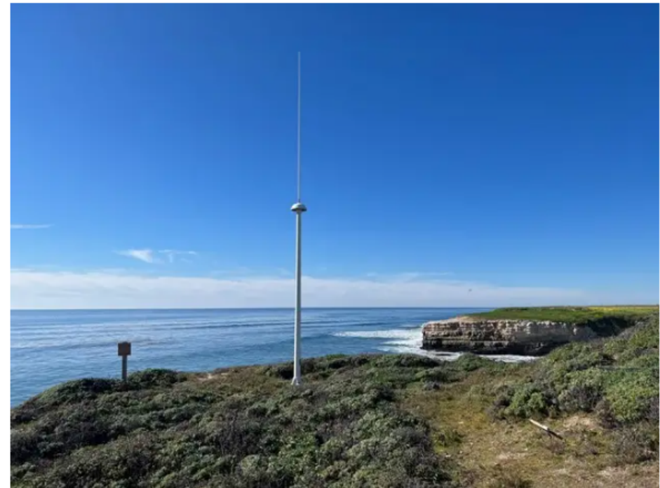
A CODAR HF radar antenna similar to the ones that will be used on the Louisiana coastline.
