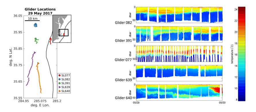
Gliders were controlled in the PEACH field experiment so that they could stay close enough together to resolve ocean fronts and eddy features. Assimilation of calculated glider team variables could be a valuable model constraint for the features that are being resolved.
