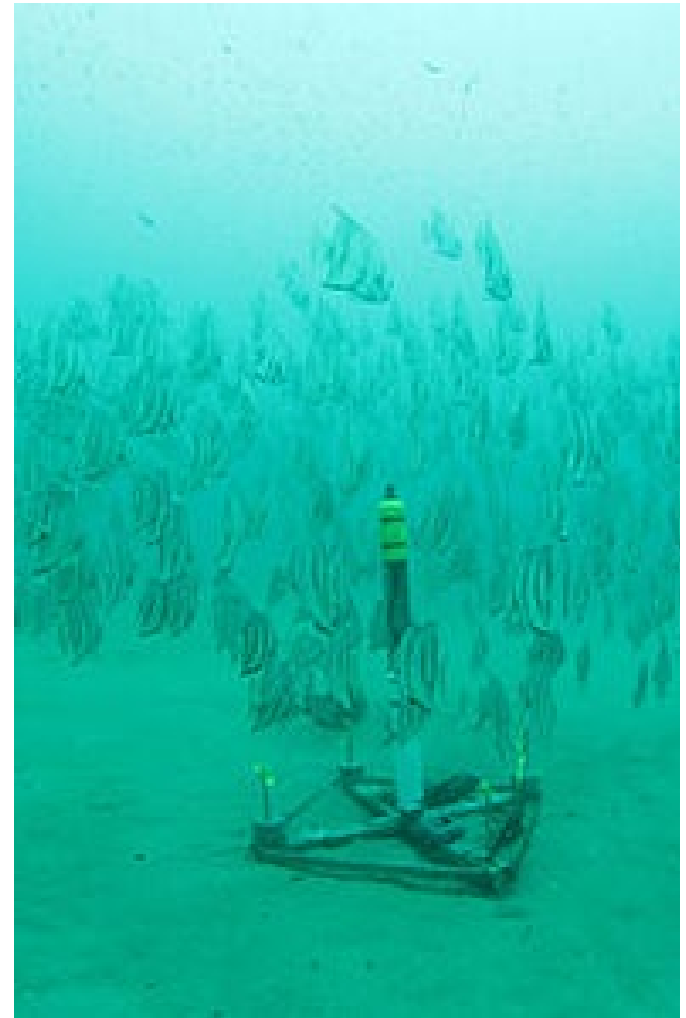
A hydrophone on the seafloor picks up signals from acoustically tagged fish. Image credit: Peter Auster/University of Connecticut
